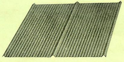
The face of the sheet is a series of shallow, parallel channels that not only stiffen the sbeet, assisting in overcoming rattling, but concentrates the water and prevents the water from being driven against the open edge of the crimp.
